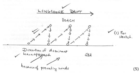
2.3.2 The sandspit across the mouth of the Umfolozi River is growing from South to North which means that the longshore drift is from south to north.
