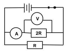
The current in the circuit is **I**. What are the readings on the ammeter and voltmeter?
