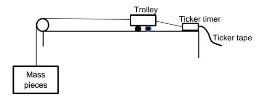
A ticker timer and tape are attached to the trolley. As the trolley moves, the ticker timer makes dots on the tape. The tape is used to analyse the motion. The learners' results are plotted on a graph as shown below.
